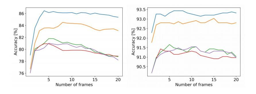
Test accuracy w.r.t. the number of image frames in the sequence shown for the proposed LprCnn-Avg/Max and the baselines SfCnn-Avg/Max/Voting.
