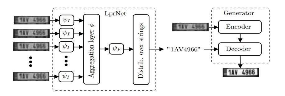
$\psi_I: X \to R^K$  and  $\psi_F: R^K \to R^D$  are CNNs with a chain architecture composed of convolution, max-pooling, fully-connected and ReLU layers
